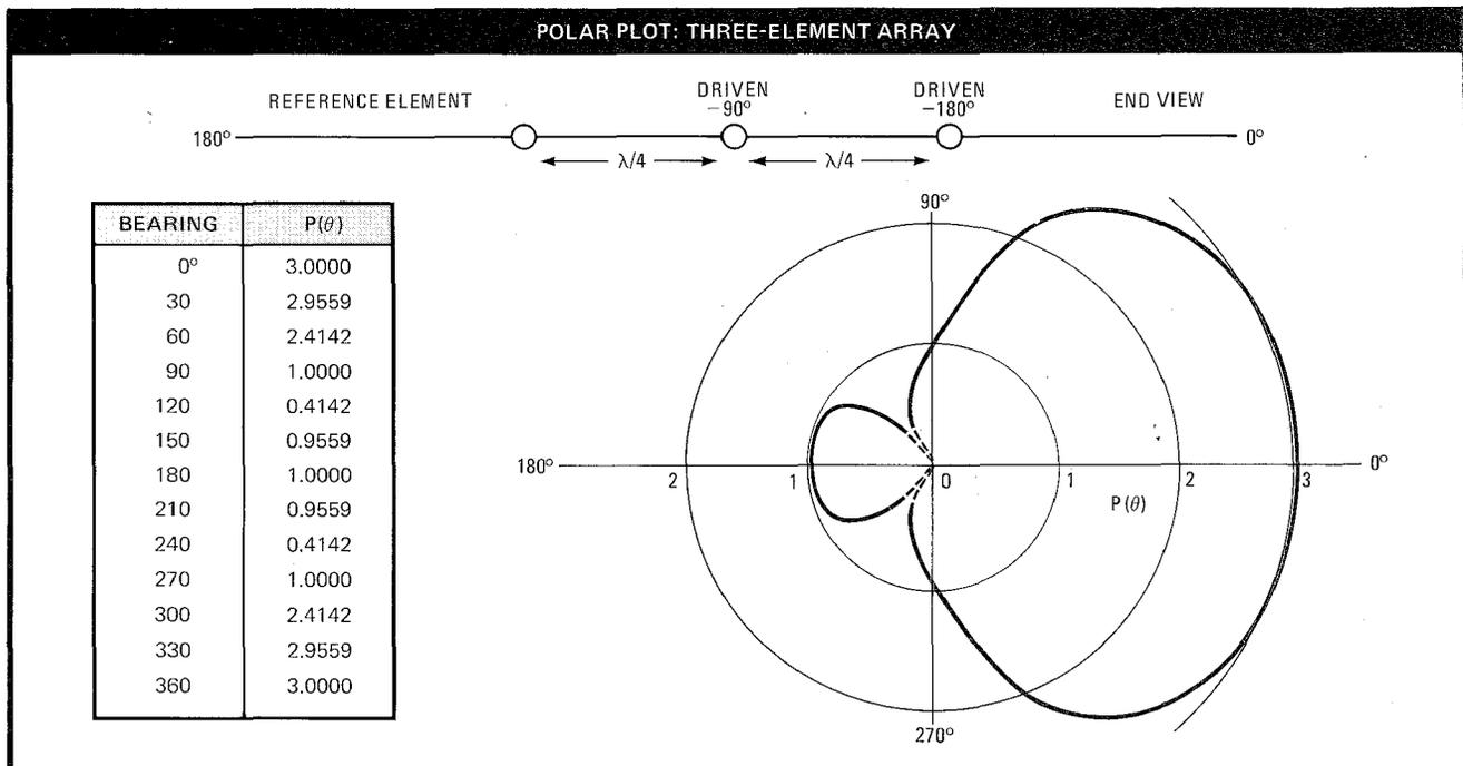
B = 180" for the third element, yields the tabulated results as shown, from which the polar plot is constructed.
